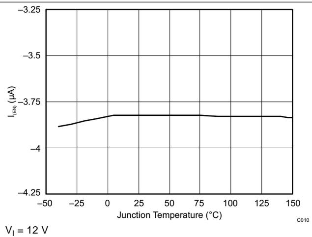
Figure 10. EN Pin Current vs Junction Temperature
