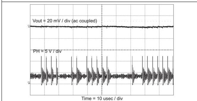
**Figure 54. Output Ripple, PSM**
