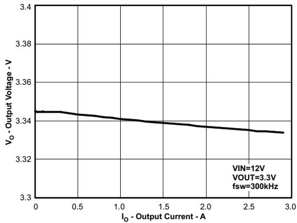
Figure 60. Regulation vs Load Current
