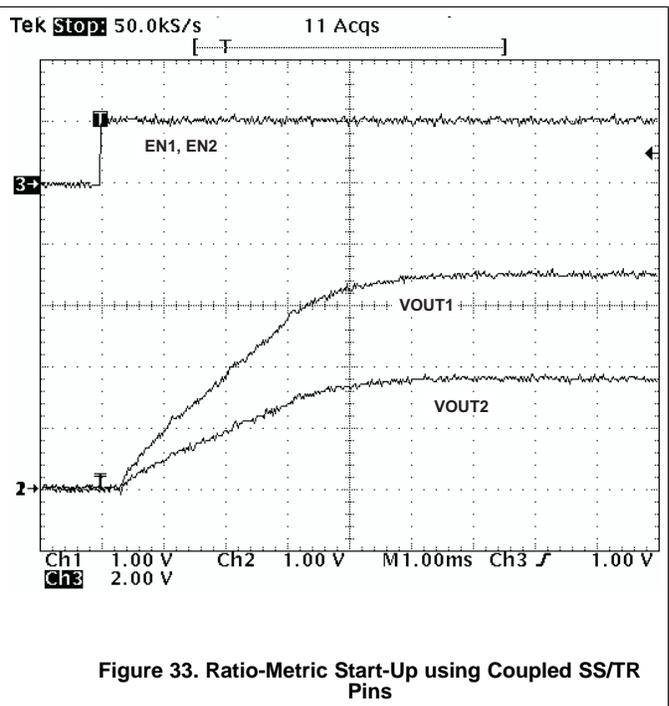
Figure 32 shows a method for ratio-metric start-up sequence by connecting the SS/TR pins together. The regulator outputs will ramp up and reach regulation at the same time. When calculating the slow-start time, the pullup current source must be doubled in Equation 6. Figure 33 shows the results of Figure 32.
