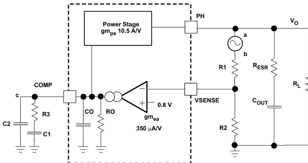
Figure 45. Small Signal Model for Loop Response
