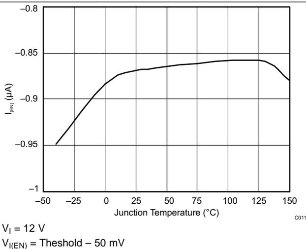
Figure 11. EN Pin Current vs Junction Temperature
