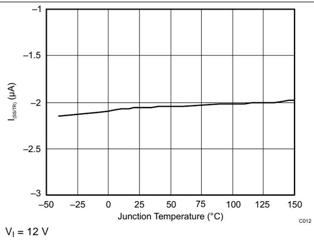
Figure 12. SS/TR Charge Current vs Junction Temperature
