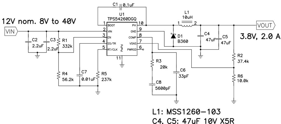
Figure 64. 12 V to 3.8 V GSM Power Supply
