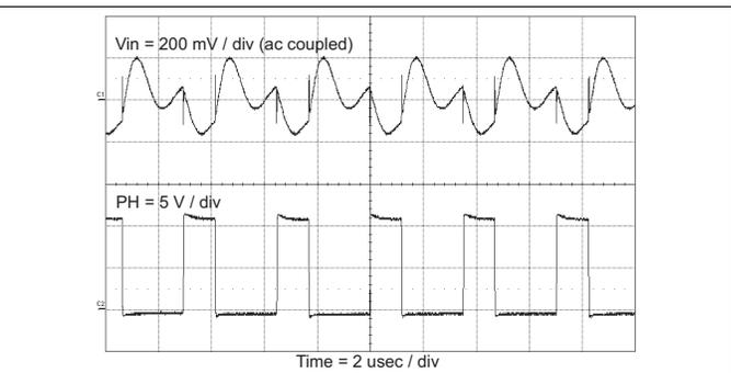
**Figure 55. Input Ripple, CCM**
