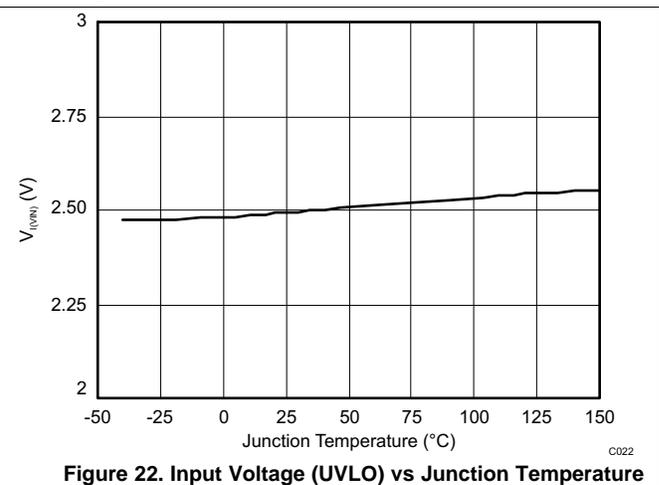
Figure 22. Input Voltage (UVLO) vs Junction Temperature
