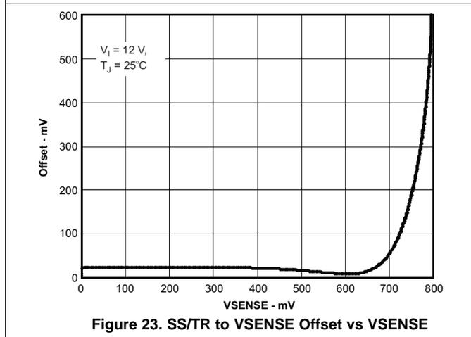
Figure 23. SS/TR to VSENSE Offset vs VSENSE
