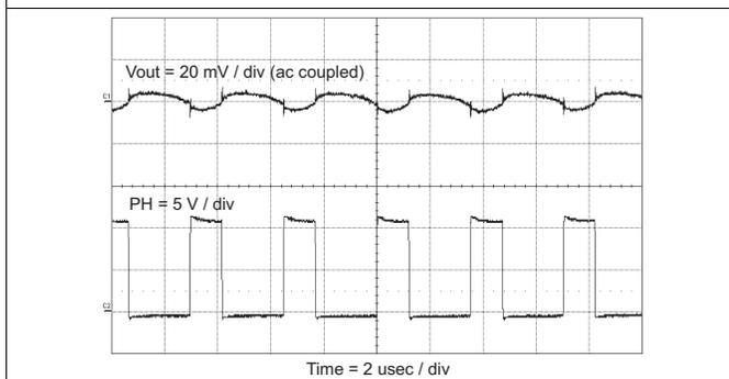
**Figure 52. Output Ripple CCM**
