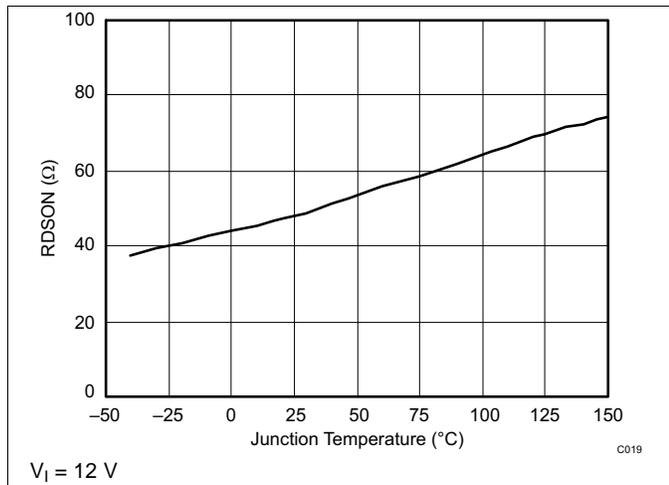
Figure 19. PWRGD On Resistance vs Junction Temperature
