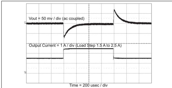
**Figure 50. Load Transient**
