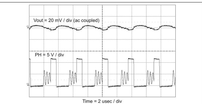
**Figure 53. Output Ripple, DCM**
