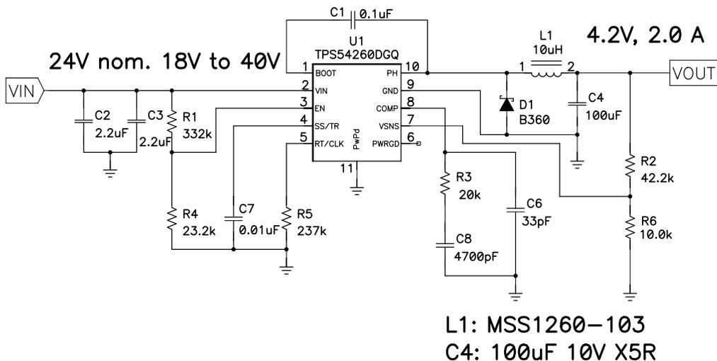
Figure 65. 24-V to 4.2-V GSM Power Supply
