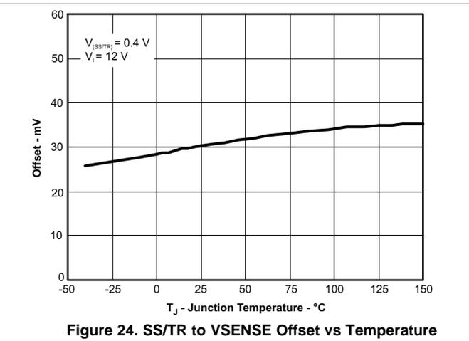
Figure 24. SS/TR to VSENSE Offset vs Temperature
