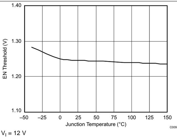
Figure 9. EN Pin Voltage vs Junction Temperature
